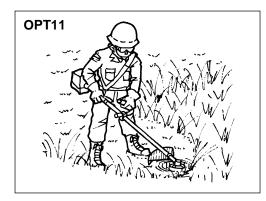
By using the shoulder strap, hang the unit on your right side. Adjust the strap length so that the cutting head may become parallel to the ground. (OPT11)
